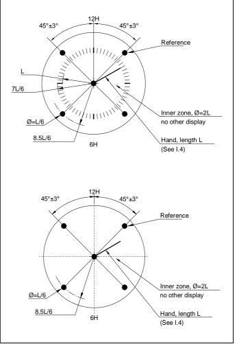
Dimensions are in mm, general tolerances  $\pm$  100  $\mu$ m, concentricity tolerance hand-axis  $\pm$  100  $\mu$ m
